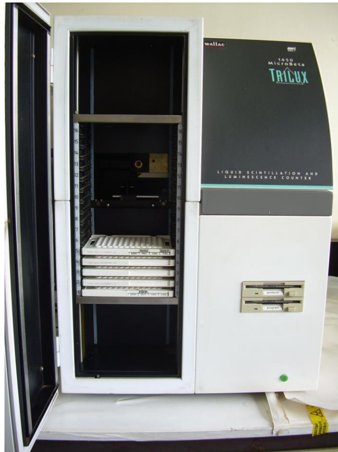
Plate 3.4: The Microbeta Trilux Liquid Scintillation and Luminescence Counter used for determination of ^3\text{H} hypoxanthine uptake by Plasmodium falciparum (D6) at the International Livestock Research Institute (ILRI) Laboratory, Nairobi. (Source: Author, 2015)
