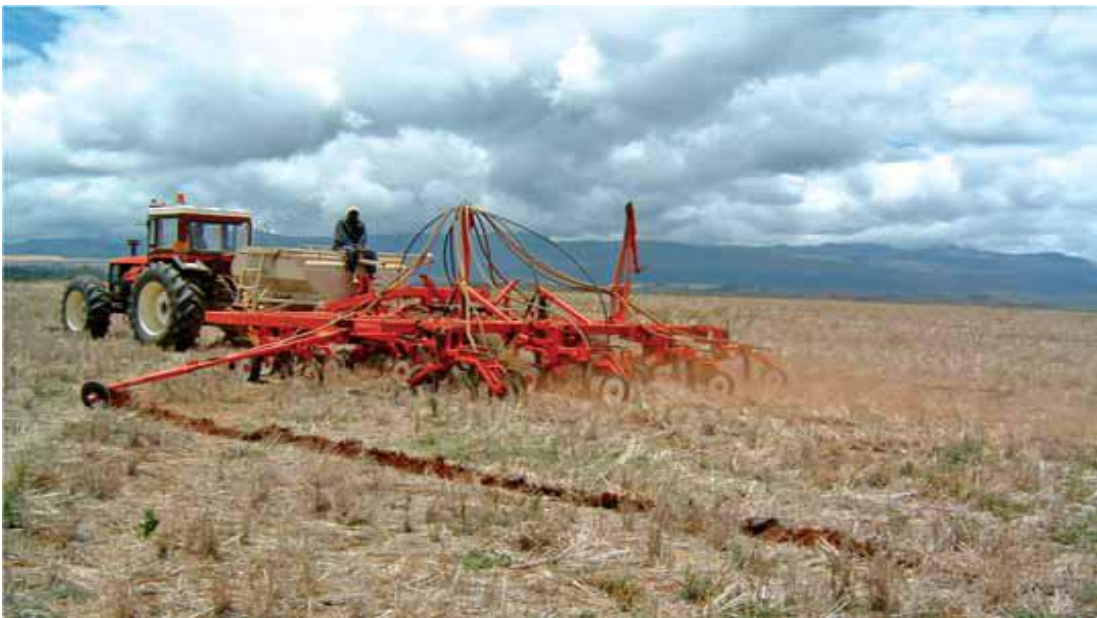
Plate D.2: Zero Tillage- Sowing operation in progress using a pneumatic seeder at Lengetia Farm Ltd. (Author, 2015)
