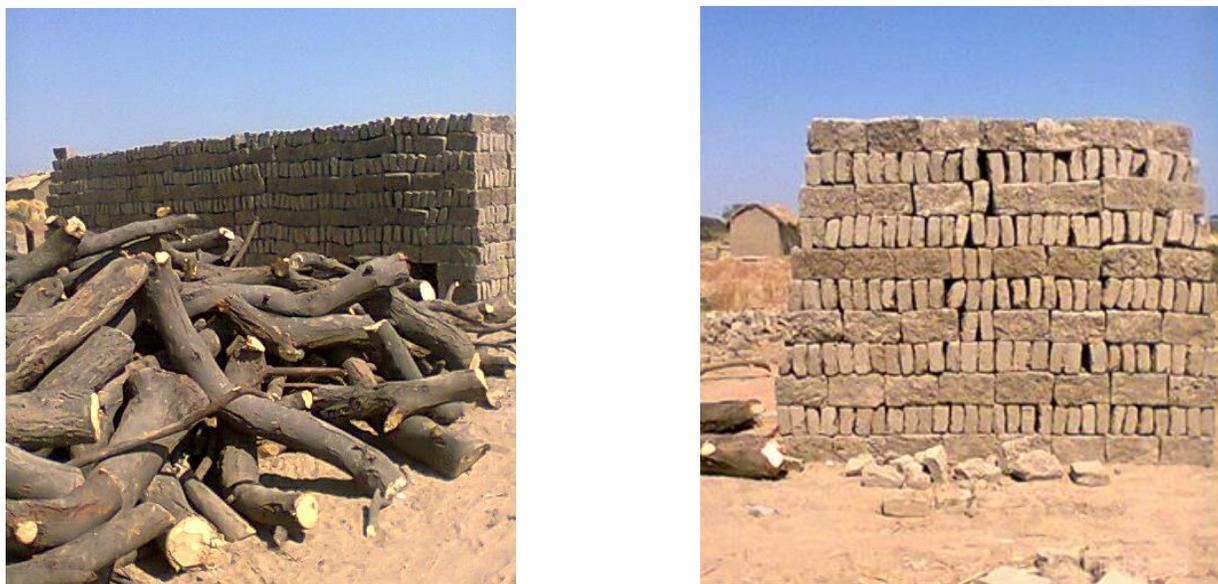
**Figure 4.2: Stock piles of bricks ready for curing using fuelwood**
