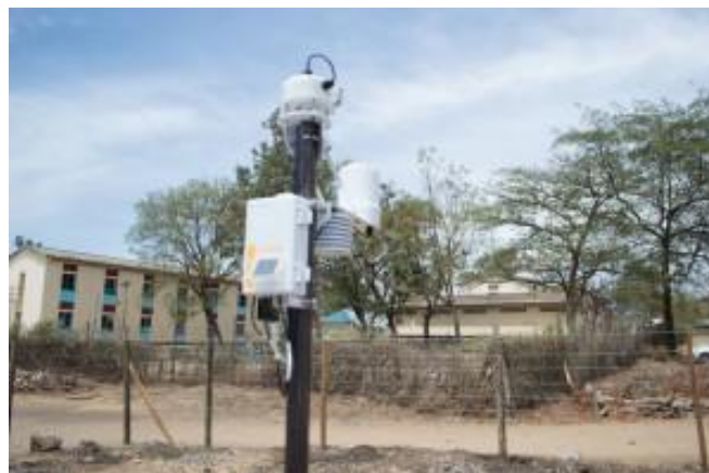
Fig. 1.2. Figure showing a weather Station installed at Homabay Kenya
