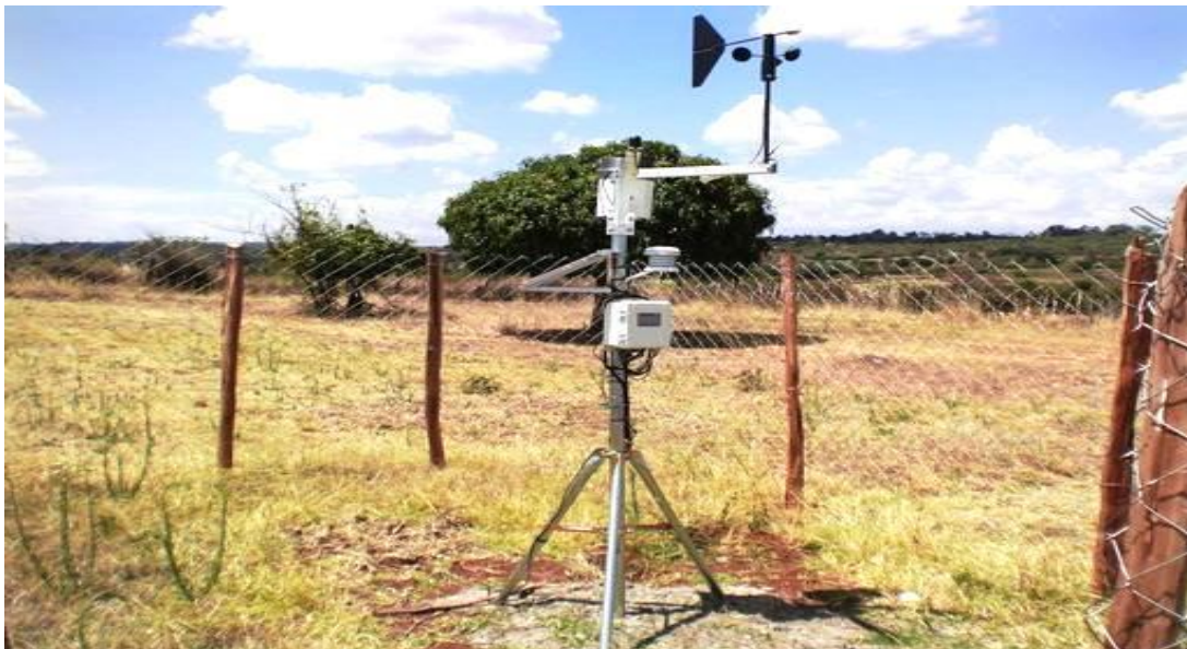
Figure 3.1: Picture of Moi University MET station showing a rotating cup anemometer used to measure wind speed ( Source: Author , 2015)
