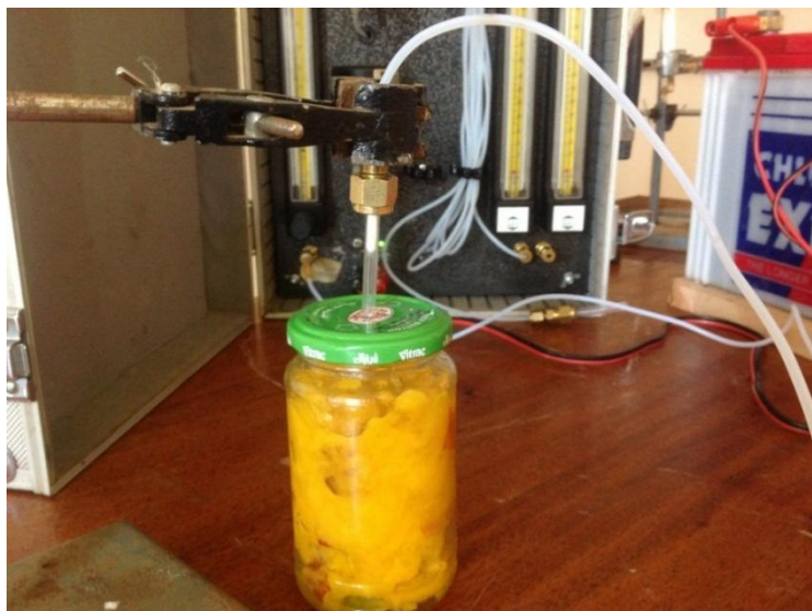
Plate 3. 2: Photo showing set up system for extraction and collection of volatile constituents (Source: Author, 2016)
