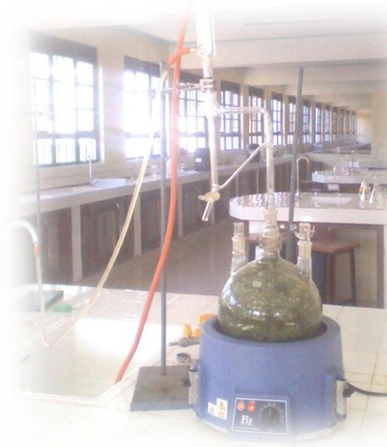
Plate 3. 1: Photo of Clevenger apparatus used in hydrodistillation of essential oils (Source: Author, 2016)
