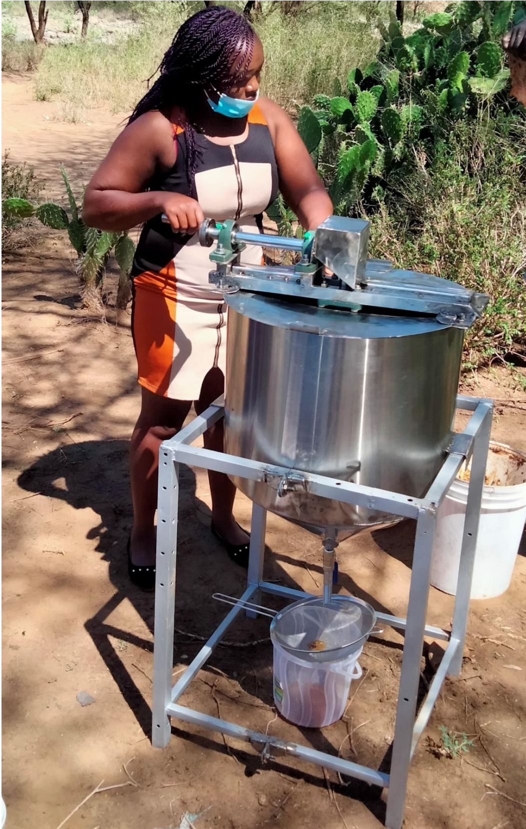
Plate 4.2: Performance test of an improved honey extractor
