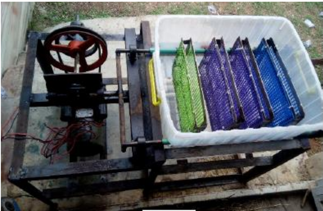
Plate 2.4: Aerial view of the vibratory honey extractor
