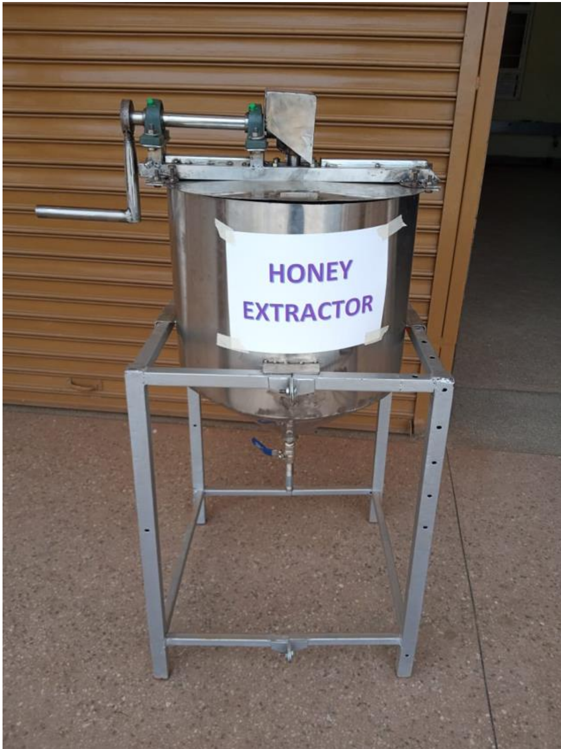
Plate 4.1: Developed honey extractor
