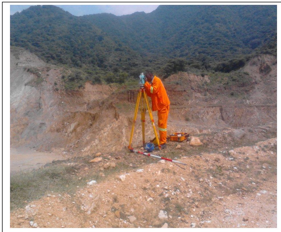
Plate 1: Total survey station on a tripod used for survey in the field. Data collected is the elevation and location points used for the calculation of area and volume (Source: Author 2013)
