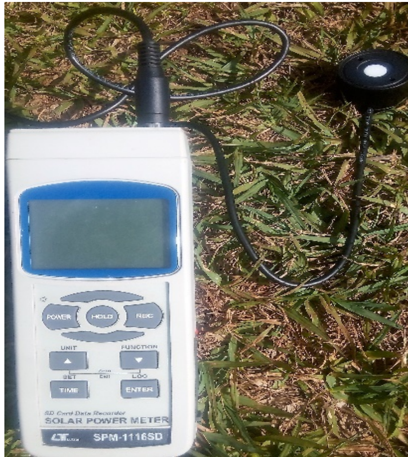
Figure 3.6: A picture of a digital recorder and the pyranometer (model SPM-1116SD)
