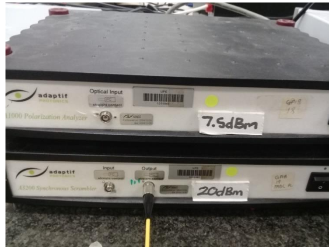
Figure 3.2: Polarization analyzer and a synchronous scrambler
