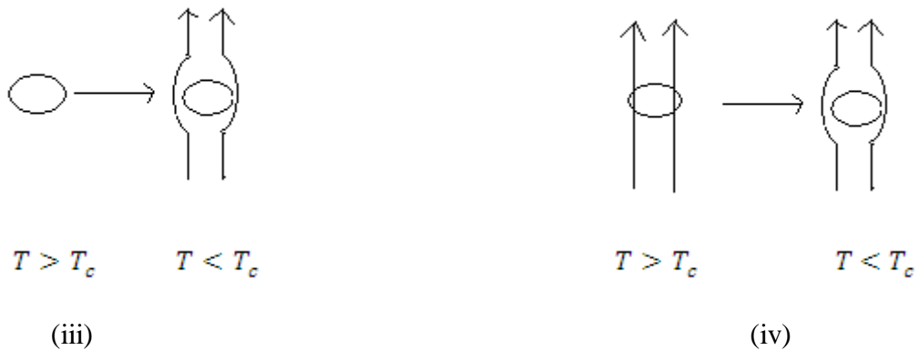
Fig 1.2 (iii): Meissner effect in type I superconductors, sample cooled below T_c before Magnetic field is applied (Meissner & Ochenfield, 1933)
