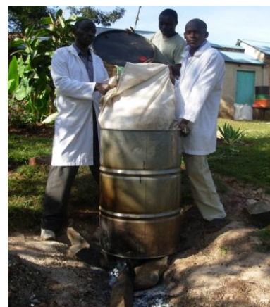
Plate 3: Pasteurization of substrates using oil drum.
