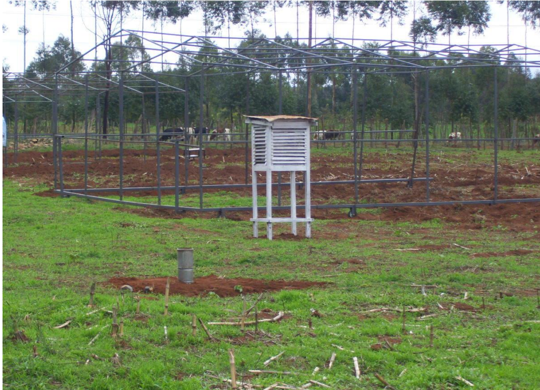
Plate 3.1: Set up of the Stevenson screen and the rain gauge at Saroiyot farm.
