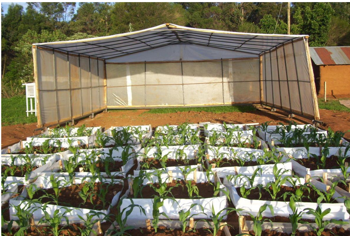
Plate 3.2: Steel frame wheeled rainfall shelter (Source: Author)
