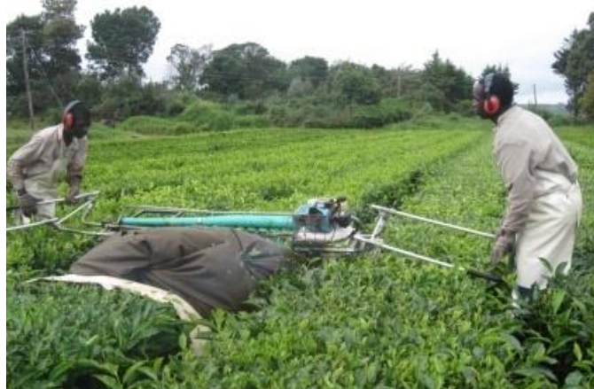
(c) Mechanical (hand held machine) harvesting method
