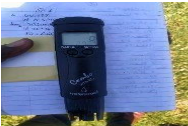
Figure 3.4: Hanna Instrument (HI) Model HI991301 equipment used for taking temperature readings
