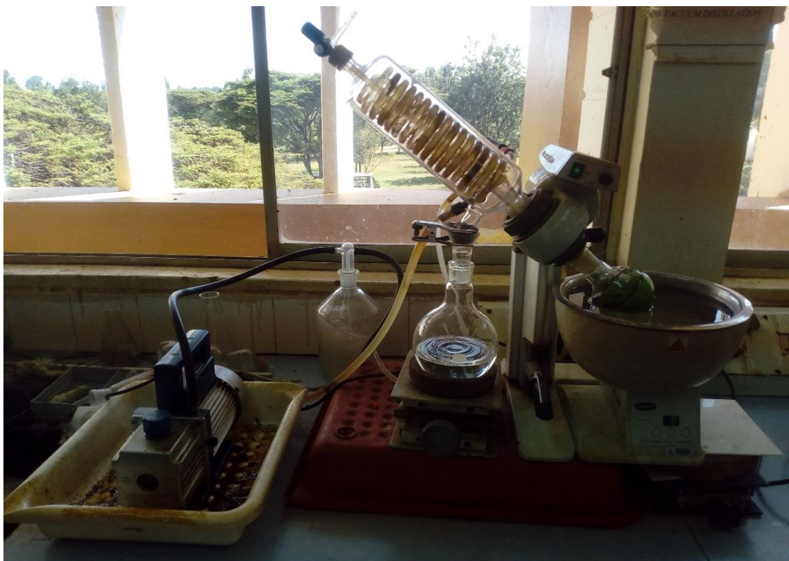
f. Concentration of extracts using a rotary evaporator
