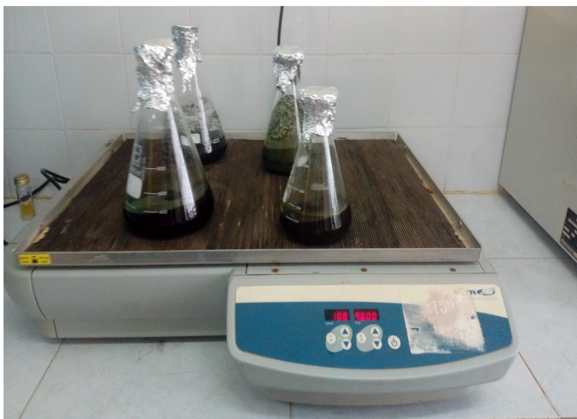
d. Agitation of plant extracts in a shaker.
