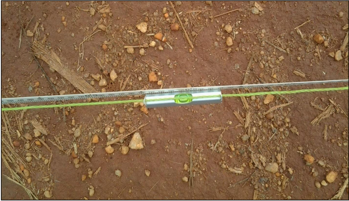
Figure 3.4: Measurement of slope using line and level. Author (Source 2013).
