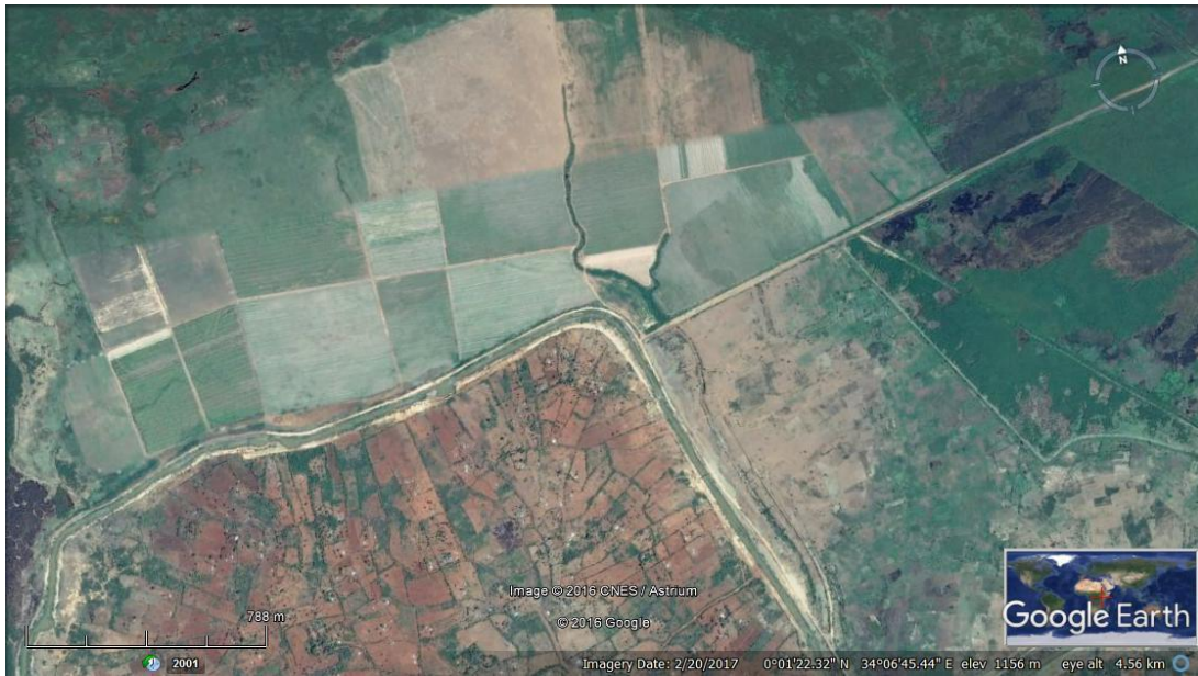
Figure 4.25: Bulungo Peninsula showing the old and current alignments of the southern canal.
