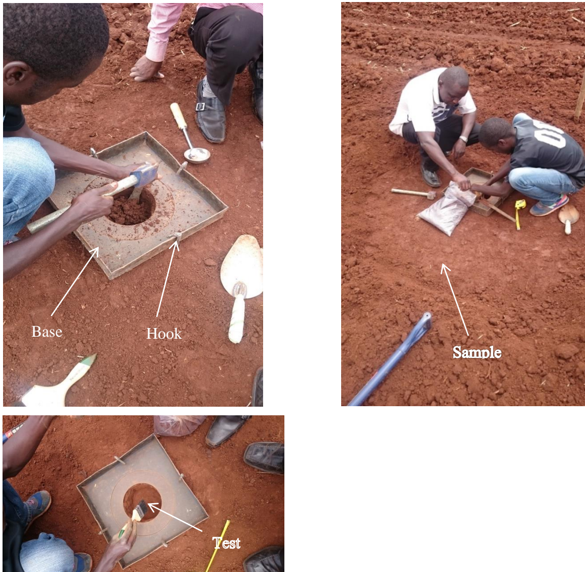
Figure 14: Preparation of the test hole ( Source : Author, 2015)
