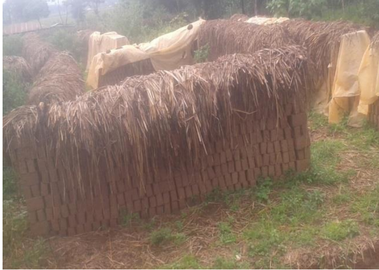
Plate 6: Bricks made using clay and covered with grass from Kingwal wetland
