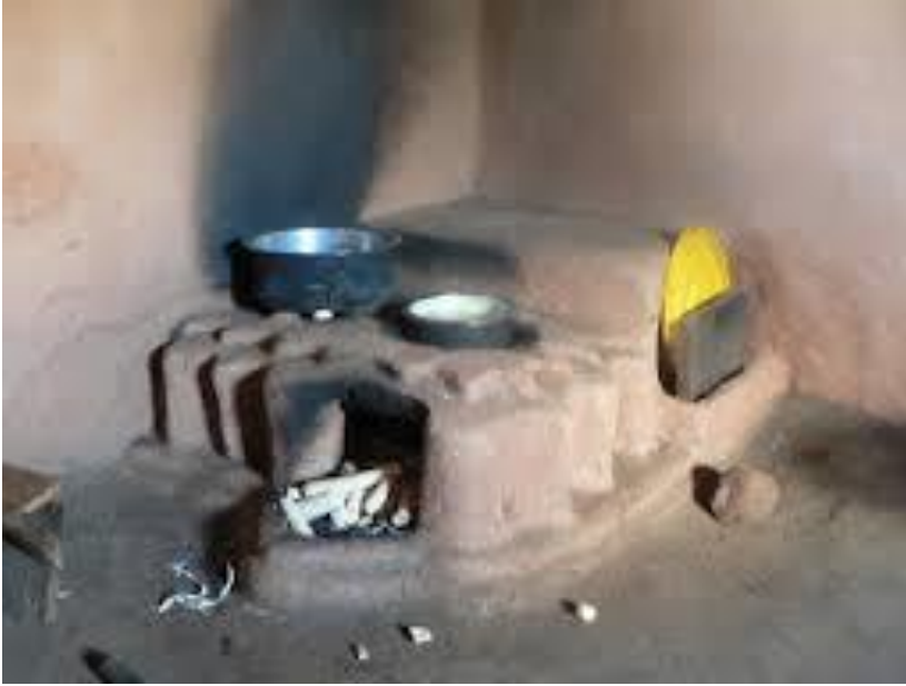
Plate 2.1: Typical Chepkube stove (Source: Allison, 2008)
