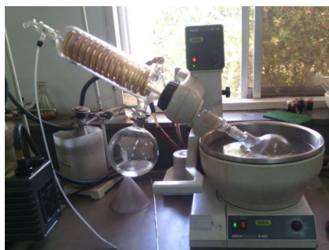
c) Removal of excess DCM and methanol using Rotor evaporator
