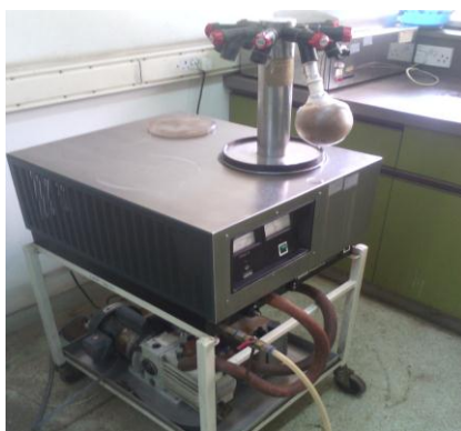
e) Extraction of aqueous extracts on freeze dryer
