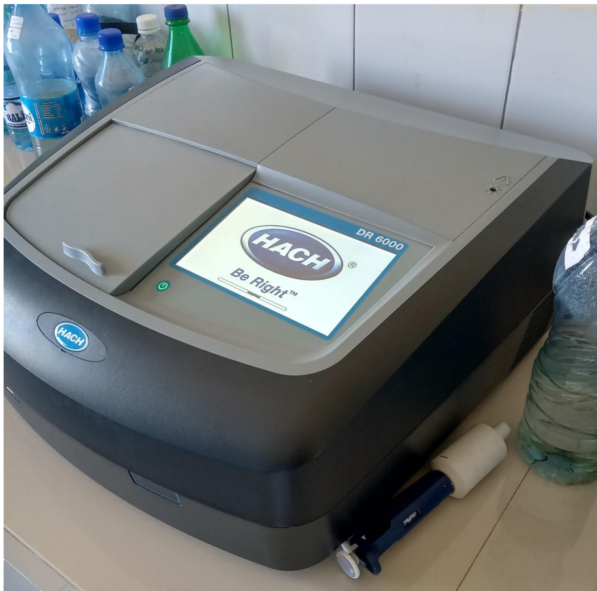
Figure 2. 2: Image of UV-Vis Spectrophotometer HACH DR6000 at ELDOWAS Laboratory
