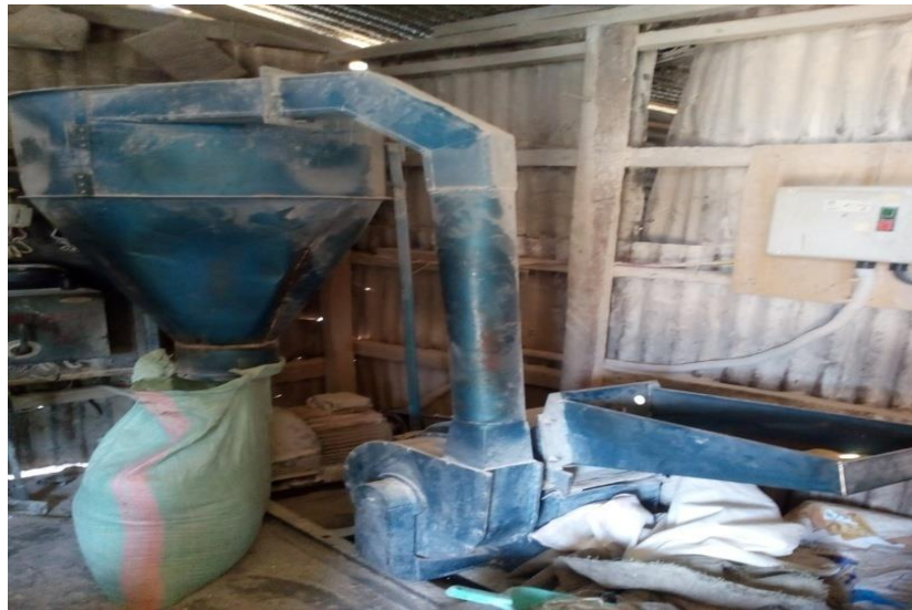
Plate 3.2: Photograph of hammer mill for grinding feed ingredients (Source: Author, 2018)
