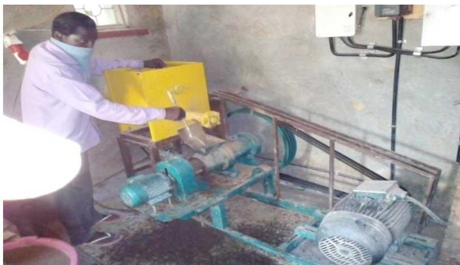
Plate 3.4: Photograph of pellet making machine (Source: Author, 2018)
