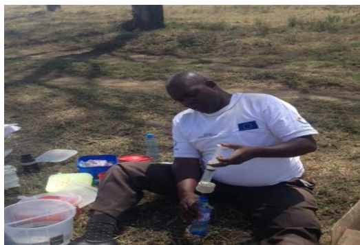
Plate 1. Filtering the water samples during field sampling.
