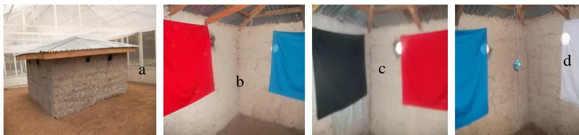
Plate 3.2 A screen house with a hut inside a); sections of hut wall with anchored fabrics inside b-d) (Source: Author, 2018).
