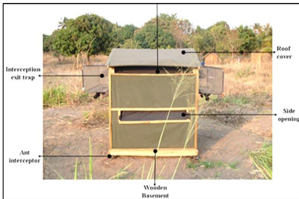
Plate 2.6 The Ifakara Odor-Baited Station (OBS); (Okumu et al., 2010).
