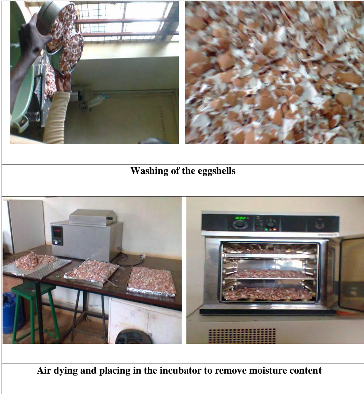
Figure 3.2 : Preparation of Adsorbent : Eggshell (Source: Author, 2013)
