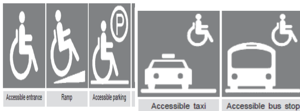
Figure 2.6: Accessibility Signs. (India Barrier Free Design Manual ,2004)
