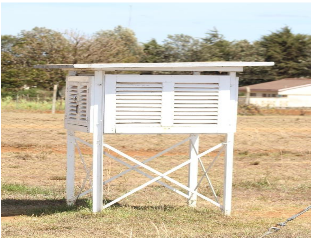
Figure 6: Stevenson screen contains four thermometers (Maximum, Minimum, dry bulb thermometer and Wet bulb thermometer).
