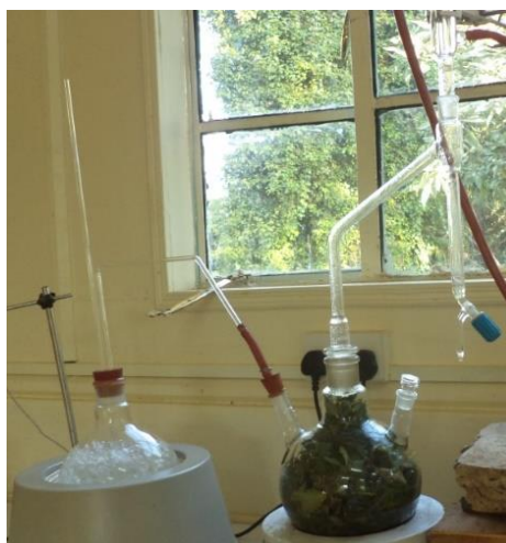
Plate 3.3: Extraction of essential oils from Ocimum species aerial parts by steam distillation
