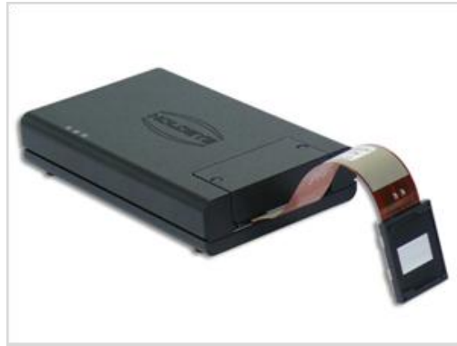
Figure 3.6: A picture of a reflective EA LCSLM manufactured by Holoeye Photonics (Holoeye Photonics, 2010). In the foreground is the LCD in which the whitish rectangular region is the active sensor area of the SLM. The black unit in the background comprises the electronics unit.
