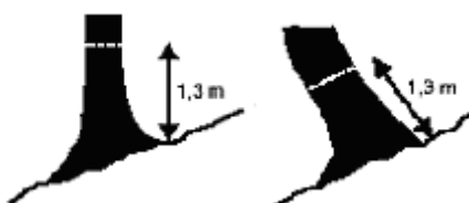
Figure 3: Diameter at breast height measurement position for a tree on steep terrain.
