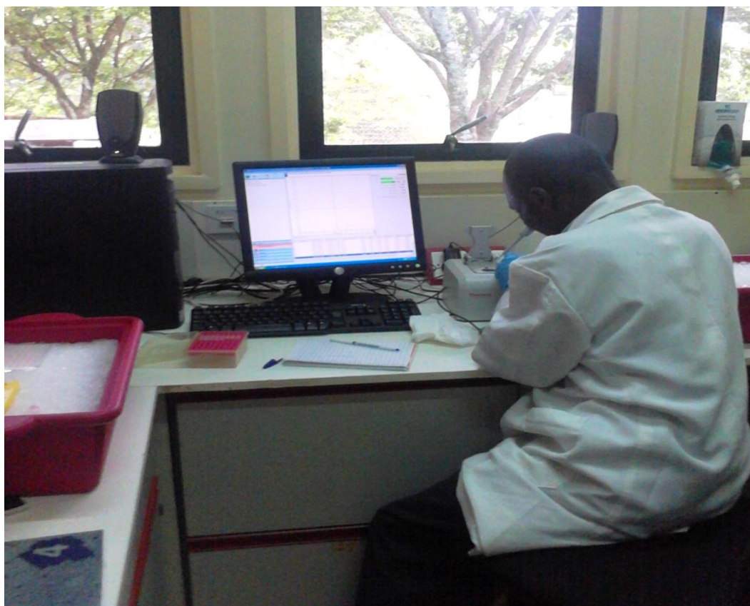
Plate 3.3: Nanodrop spectrophotometry. It was used to check whether the Qubit ® readings were reliable (Source: Author).
