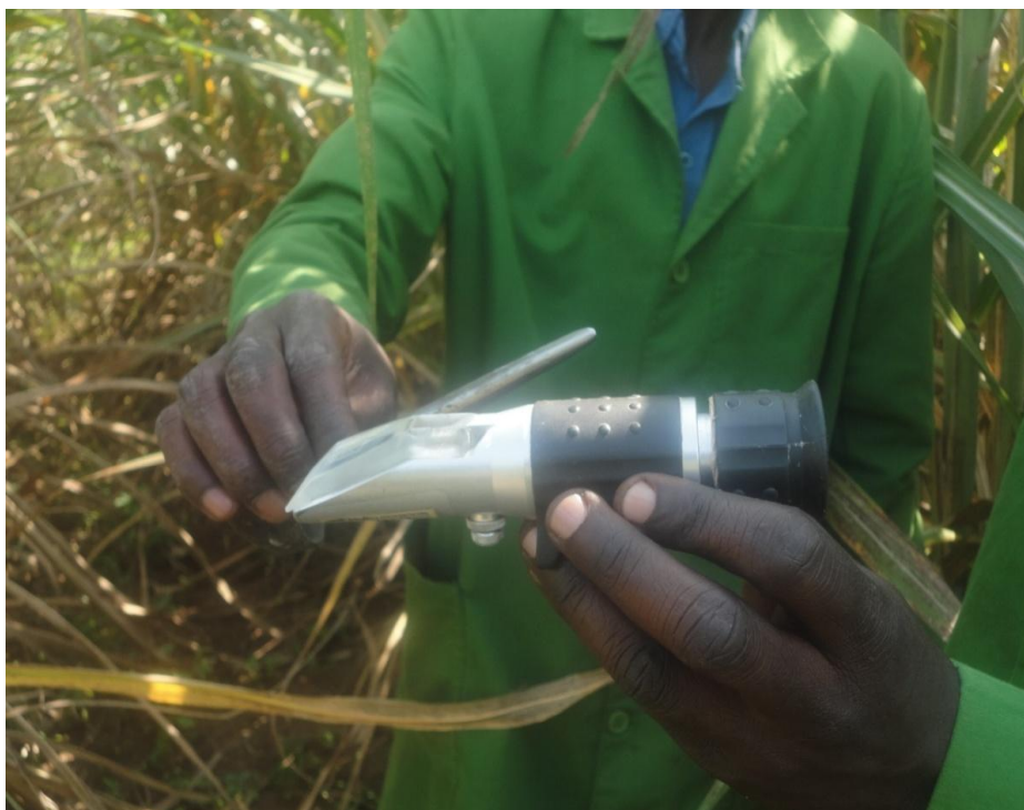
Picture showing quality assessment using hand refractometer
